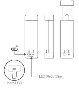
A. Connecting: Plug one end of the included Micro USB cable into the input port and the other end into a power supply (adapter, PC or other standard USB output port). Upon powering up, the LED will light up.
